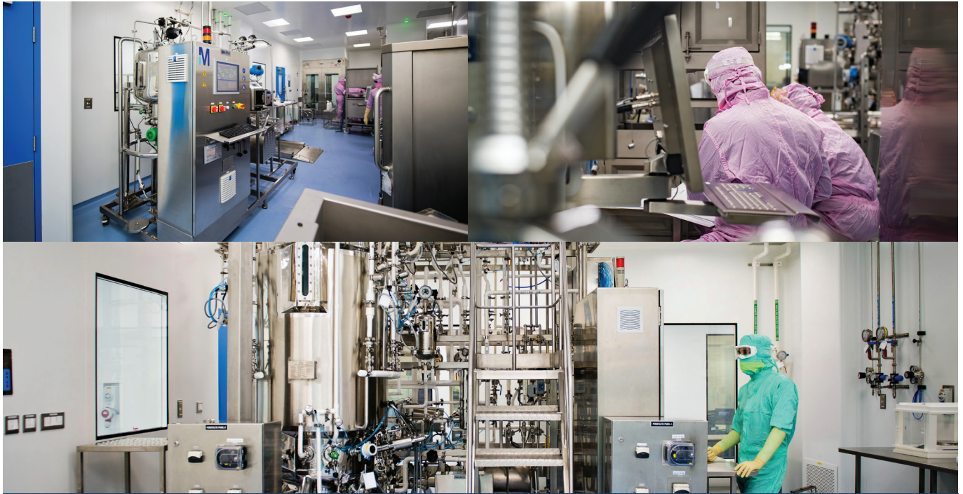
Figure 5: Manufacturing workflow in our dedicated microbial facility from counterclockwise: SS microbial fermenter, AKTA chromatography system, and automated tangential flow filtration system.
