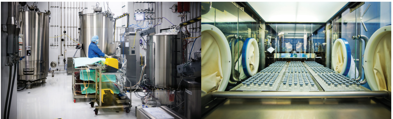
Figure 6: Our dedicated Biologics (mammalian) manufacturing facilities, with our single use bioreactors and an isolator line for fill and finish
